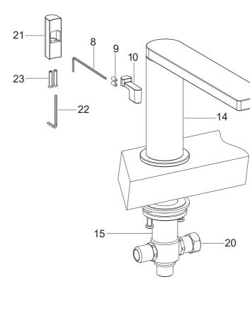
\*\*Color code must be specified when ordering. **NOTE:** For all Asia pacific regions (excluding China) add SP (SPxxxxxx\*\*) in front of the part number when ordering. Slide the o-ring(17) into the bottom groove of the escutcheon(16). Tighten the escutcheon with the o-ring onto the diverter kit(15), and keep it against the bath tub. Position the diverter kit so that the nut(20) is on the right. Screw the nut(18). Tighten the screws(19) to secure the diverter kit.
